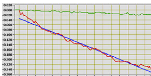
Time profiles of a test sample stored at 40°C/dry (green) and 40°C/75% relative humidity (red). Blue line: calculated linear regression of the 40°/75 % r.h. sample. X-axis: Storage time [day]. Y-axis: Calculated scores.
